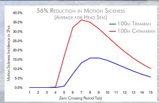
\*Note: All seakeeping data for vessels with 340 tonnes deadweight @ 37 knots in 2.5 metre seas (significant wave height).
